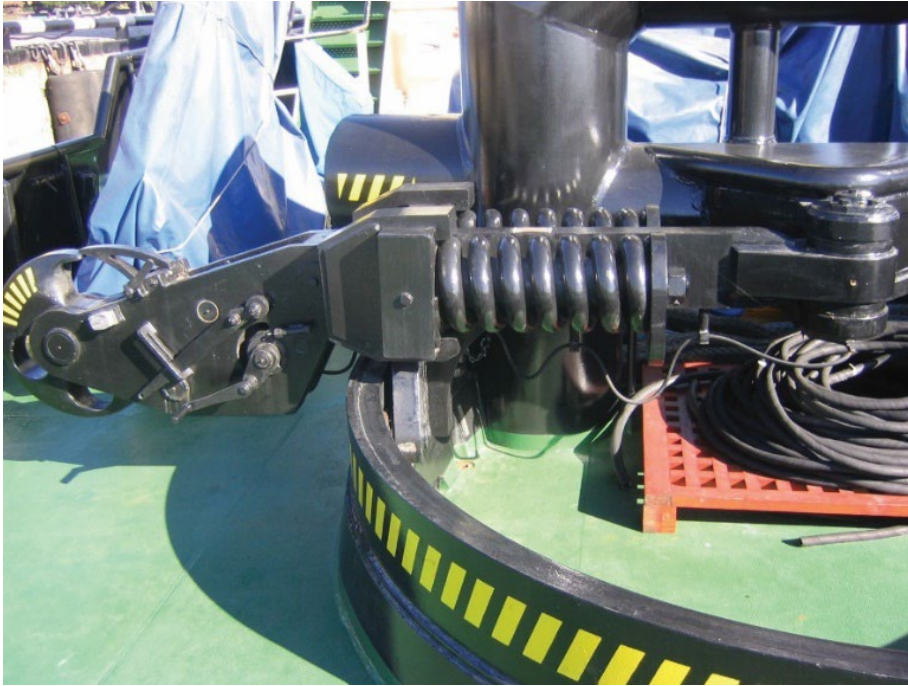
Figure 4 Tug with radial towing hook
